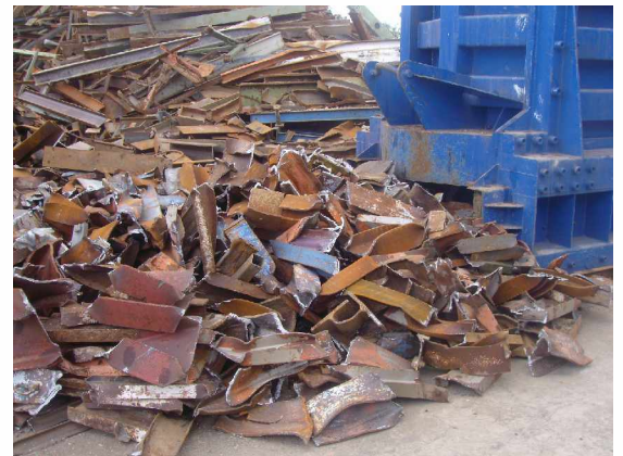
Pic. 3: sheared cupola scrap sorting on the front discharge
